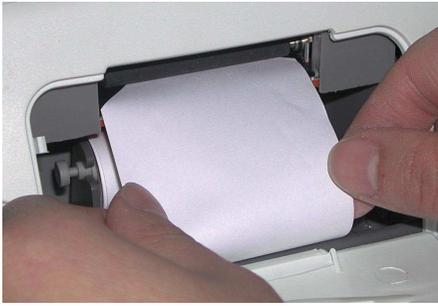
Press S/L to roll the paper to 2cm, and press to stop
